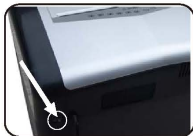
Main Power Switch
