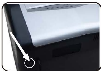
Main Power Switch
